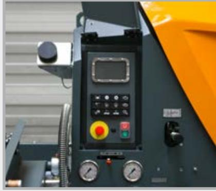
The central control panel with intuitive keypad increases operating safety. A transparent display supplies the user with all relevant information.
