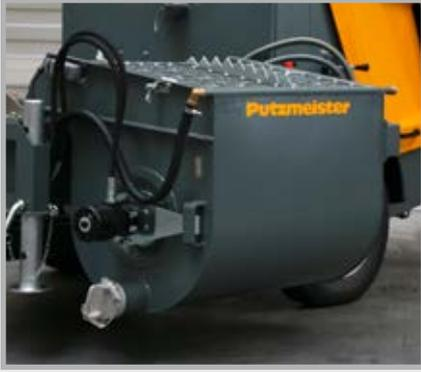
The large mixer with 240 l volume and integrated water dosing tube makes possible the mixing of larger material quantities on the construction site, e.g. EPS container in 200 l bags.
