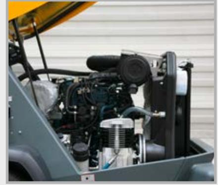
The powerful diesel engine with 28 kW and diesel particulate filter complies with the requirements of the exhaust emissions standard „Stage V“. The air required for spray applications is provided by the compressor.
